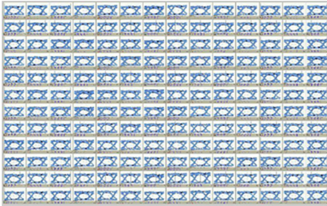
Fig. 4. PRBS31 eye diagrams from a 12 \times 14 VCSEL matrix at 8 Gb/s line-rate [26].
