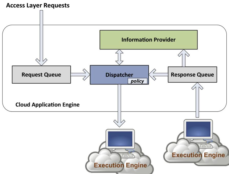
Fig. 7. Cloud application engine components.
