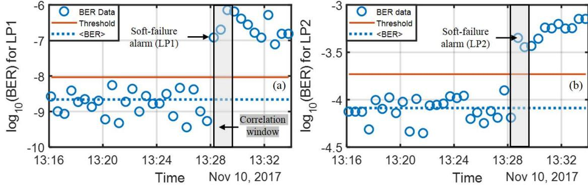
Figure 6. BER vs time for LP1 (a) and LP2 (b) for the emulated soft-failures on Link<sub>1-2</sub>.
