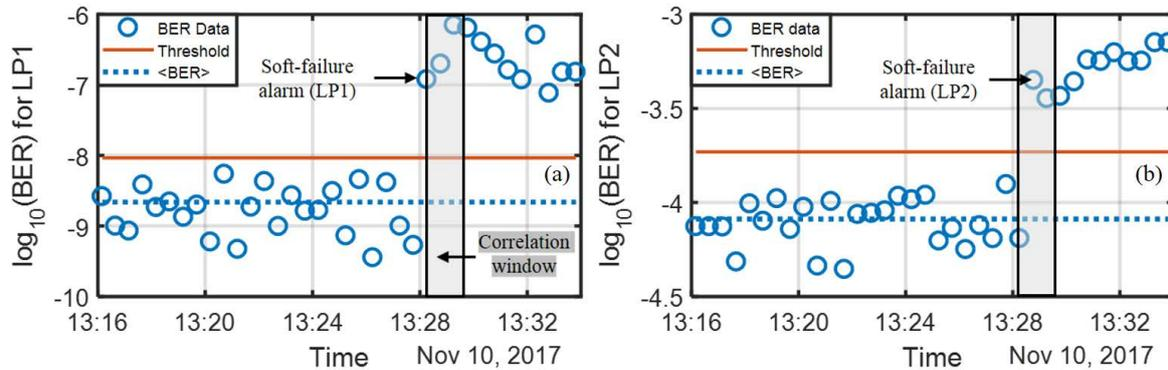
Figure 6. BER vs time for LP1 (a) and LP2 (b) for the emulated soft-failures on  $\text{Link}_{1,2}$ .
