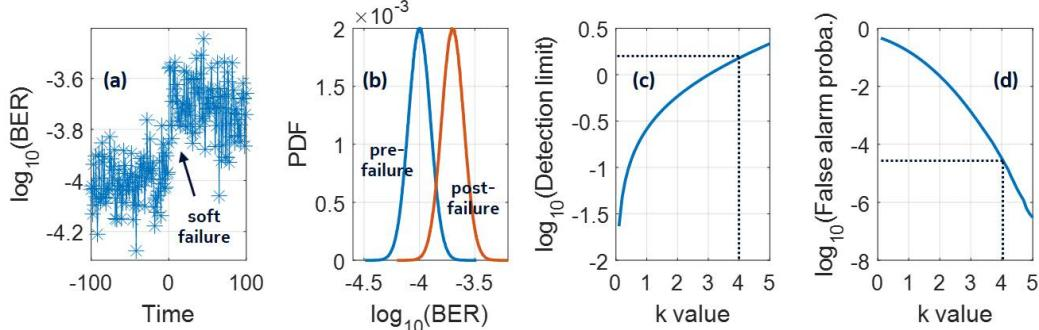
Figure 2: (a) Simulated evolution of BER over time with soft-failure; (b) Probability density function (PDF) of BER before and after the soft-failure; (c) Soft-failure detection limit (c) and false alarm probability (d) versus  $k$ .
