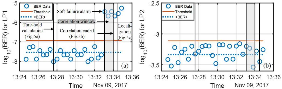
Figure 4. BER vs time for LP1 (a) and LP2 (b) for the emulated soft-failures on Link<sub>0-1</sub>.
