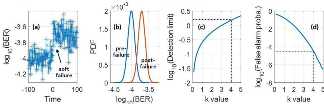
Figure 2: (a) Simulated evolution of BER over time with soft-failure; (b) Probability density function (PDF) of BER before and after the soft-failure; (c) Soft-failure detection limit and (d) false alarm probability versus  $k$ .
