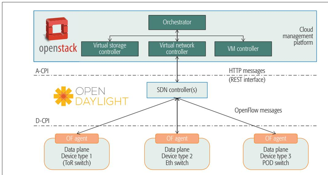
Figure 5. Overall architecture of the NEPHELE data center control infrastructure.
