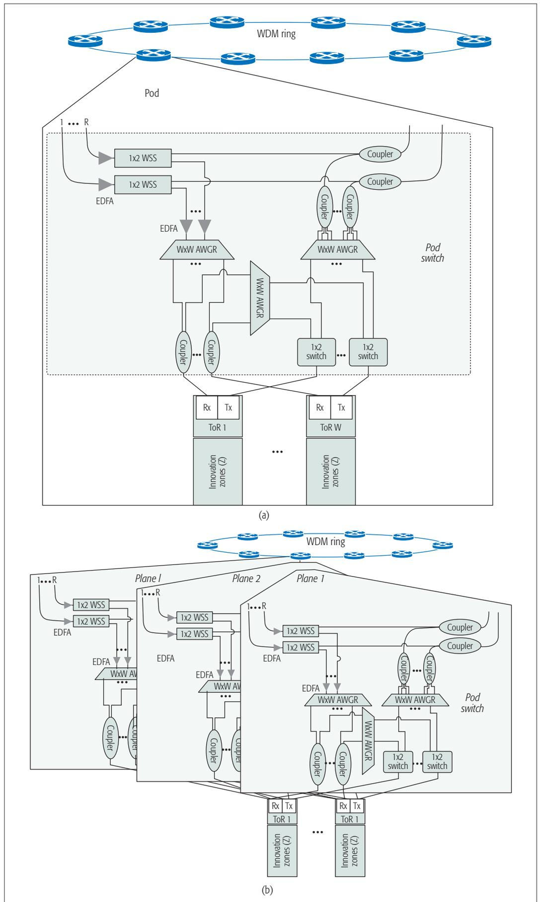
Figure 1. a) The NEPHELE optical data center network architecture; (b) scaling the NEPHELE network with the addition of optical planes.
