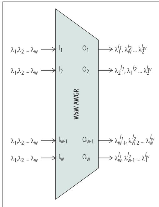
Figure 3. AWGR's routing characteristics.
