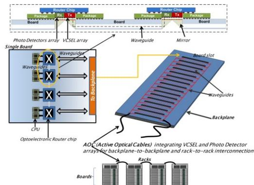
Figure 1: Illustration of the application of photonics in “in-the-box” networks: AOCs, Optical Printed Circuit Boards, Opto-electronic chips.
