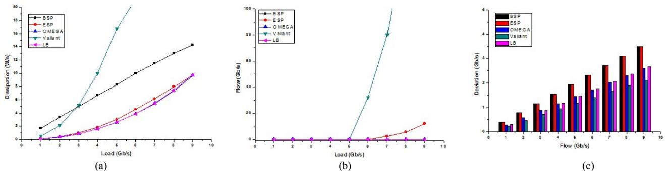
Figure 5: Total network (a) energy dissipation, (b) flow losses and (c) standard link load deviation of the 4x4 Mesh topology over SuperLU.
