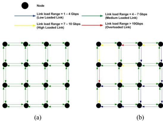
Figure 4: Link loads for (a) OMEGA and (b) shortest path
