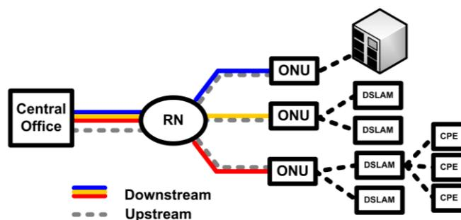
Figure 1. The proposed multi-wavelength PON architecture.
