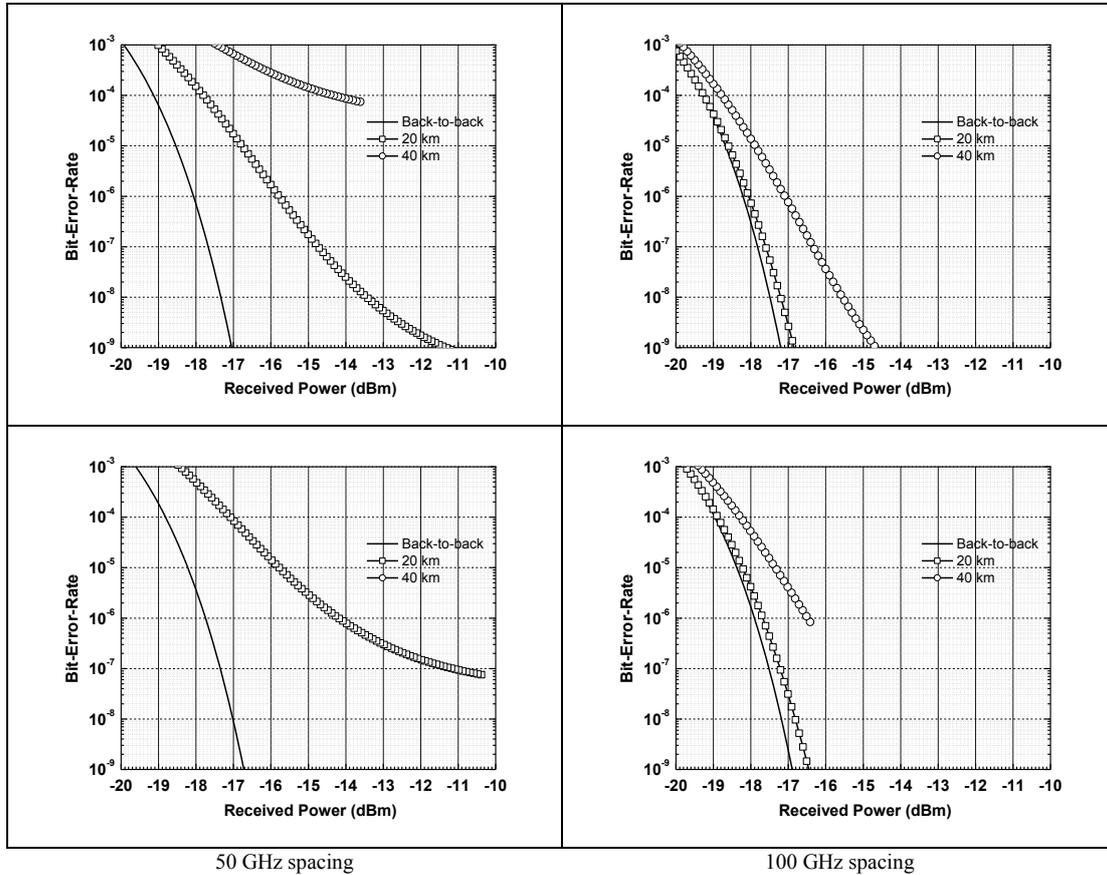
Figure 2. Physical layer performance evaluation for the splitter-based PON architecture. The number of wavelengths equals 64 (top row) and 128 (bottom row).
