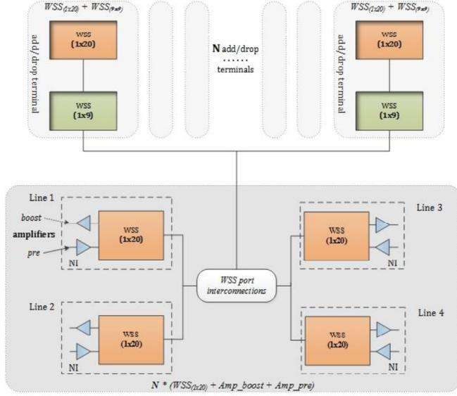
Fig. 1. Colourless, directionless, and incrementally contentionless node architecture.
