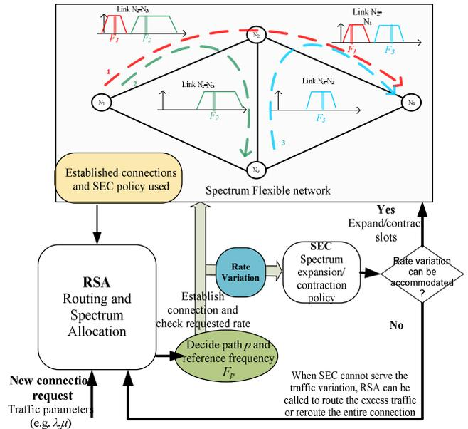
Figure 3: Flow diagram of a generic approach to operate a flexible network.
