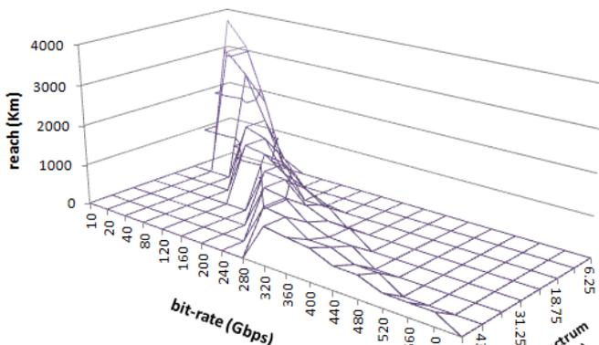
Figure 1: Transmission reach as a function of the rate and spectrum used for a specific flexible transponder.
